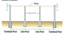
Dig line post holes approximately 6" in diameter and 18" - 24" deep. The exact diameter and depth will be determined by local conditions.
