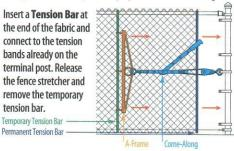
Fasten the fabric securely with Fence Ties spaced approximately 24" along the top rail and 12" on each line post. Finally, securely tighten nuts on all rail end bands and tension bands.
